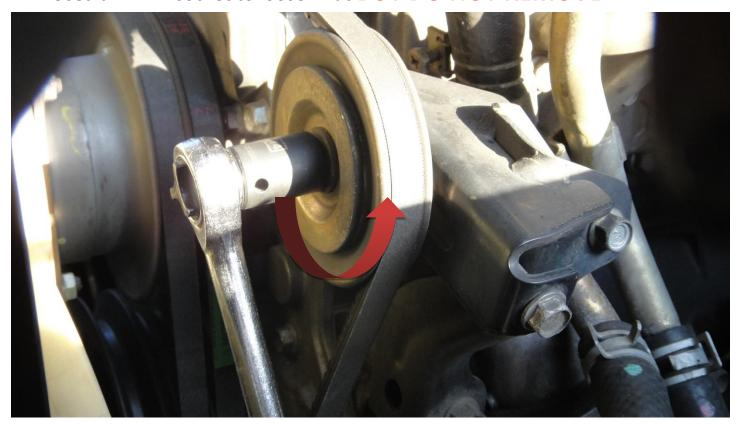
3. Use a 12mm socket. Turn the socket in increments of ½ turn to the right
