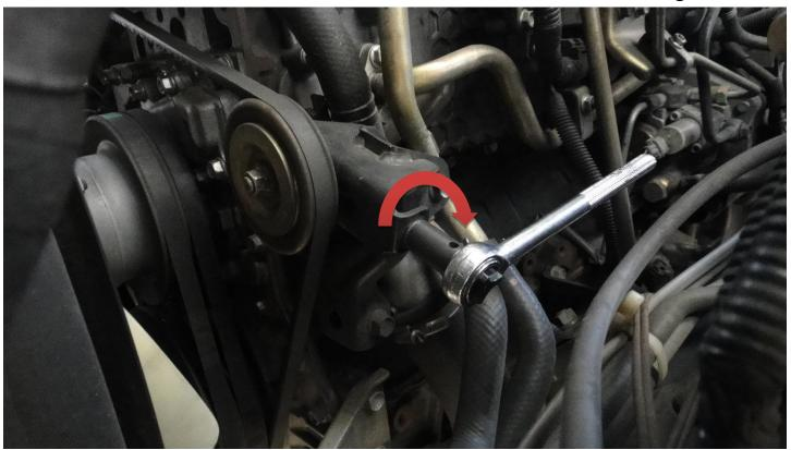
Check the tension adjust if necessary but don't over do it
