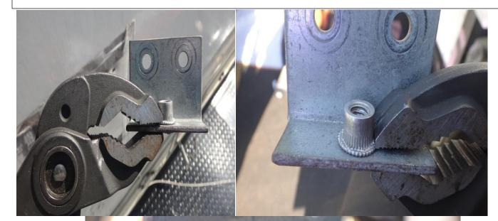
Using Channel lock pinch the edges as in photos. For a better hold use krazy glue for metal
